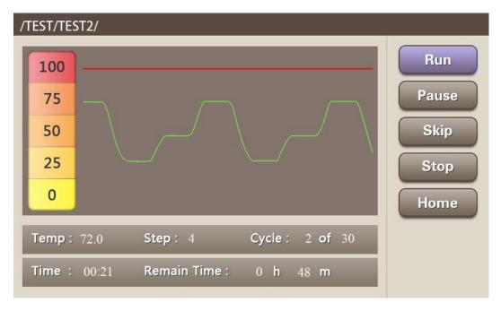
When the heated lid reaches the setting temperature, the program starts to run.
